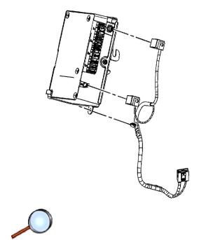
4. Disconnect the VCIM electrical connectors as necessary.
