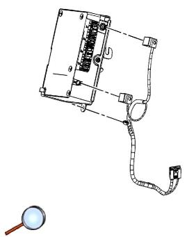
3. Connect the VCIM electrical connectors as necessary.
