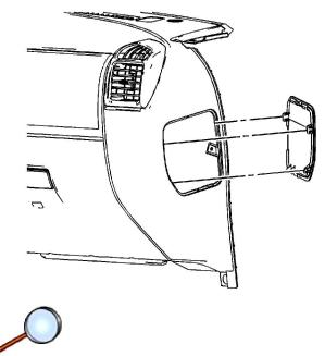
3. Remove the service panel located on the right side of the instrument panel (I/P).
