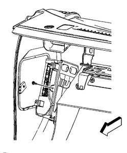
5. Remove the screw retaining the VCIM to the bracket.
